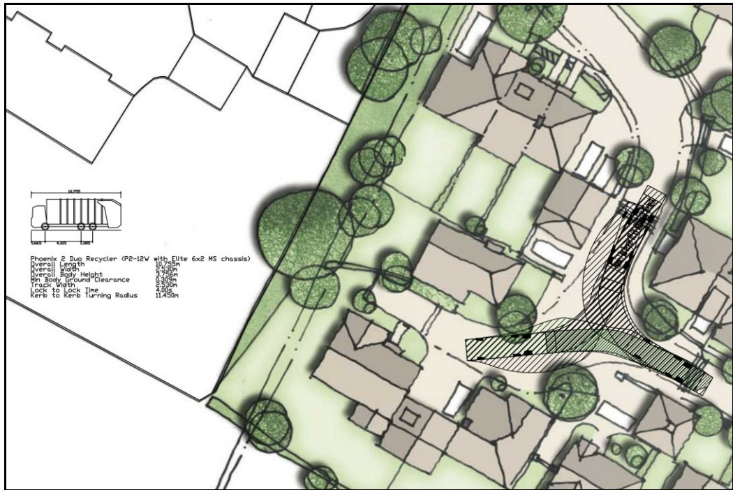
Figure 15. Swept path analysis, turning.
