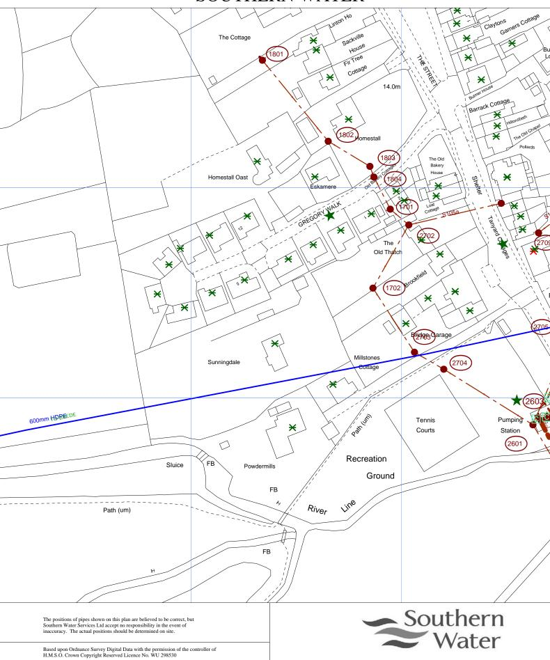
Scale: 1:1250 O.S. REF: TQ7817NW Screen Print WARNING: BAC pipes are constructed of Bonded Asbestos Cement WARNING: Unknown (UNK) materials may include Bonded Asbestos Cement
