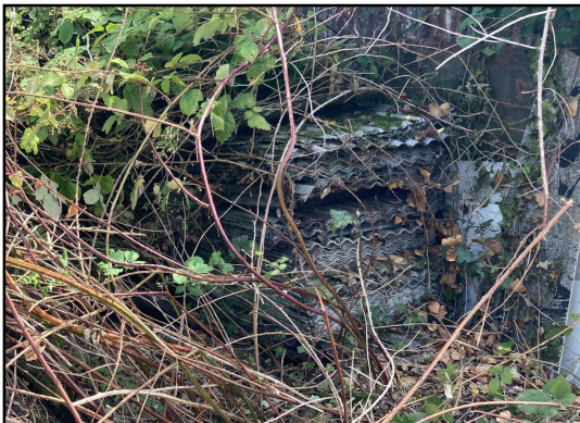
Plate 23. Stack of corrugated sheeting, potentially containing ACM, in the west of the Site
