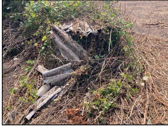
Plate 26.. Stack of corrugated sheeting, potentially containing ACM in the center of the Site
