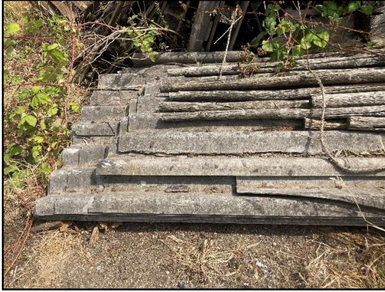
Plate 25. Stack of corrugated sheeting, potentially containing ACM in the center of the Site.
