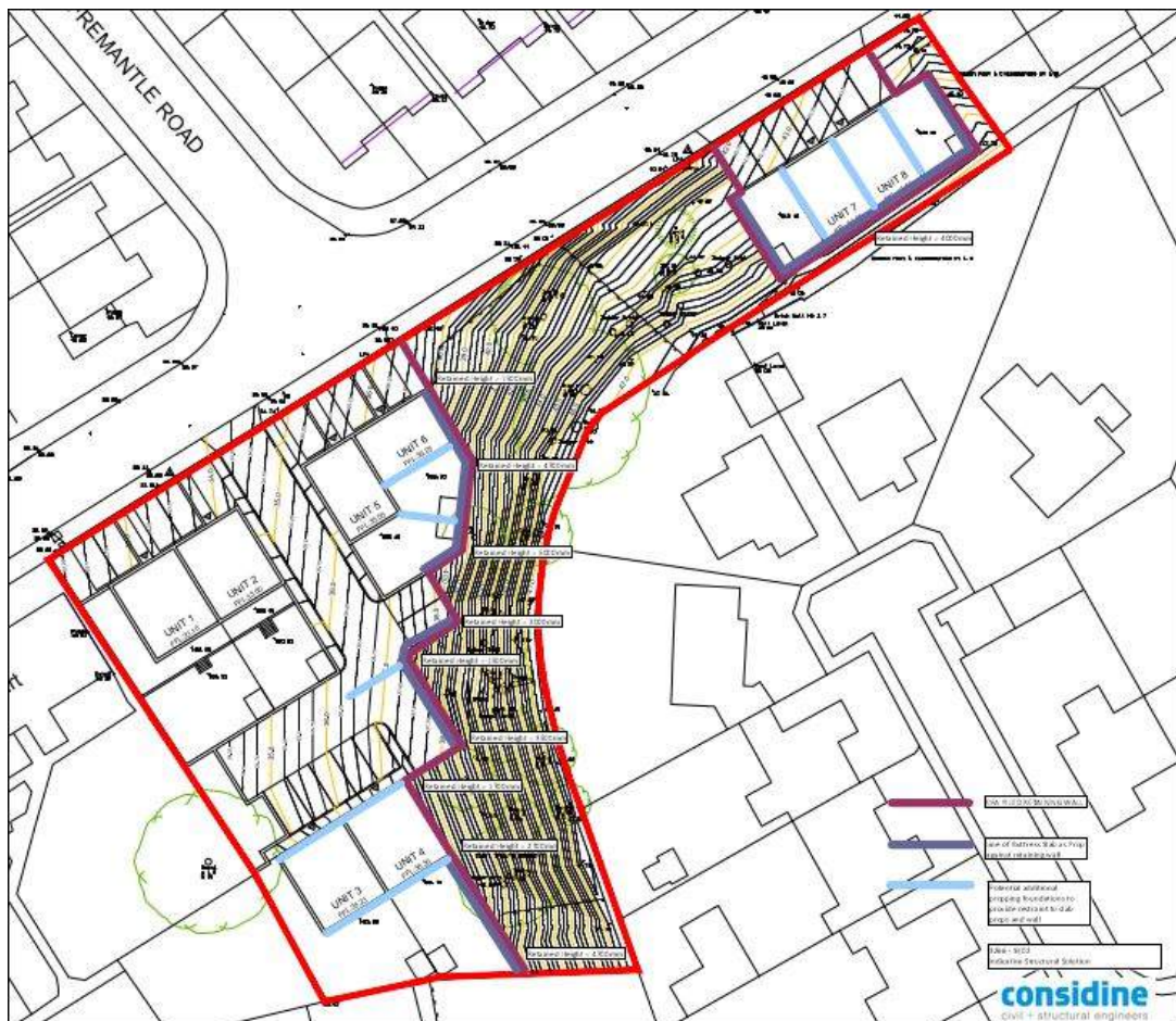
Figure 3.2 – Example of a retaining wall solution - Layout
