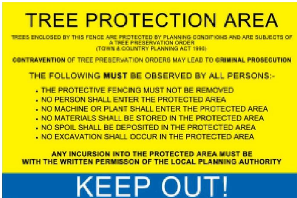
Figure 12 Example of warning signs
