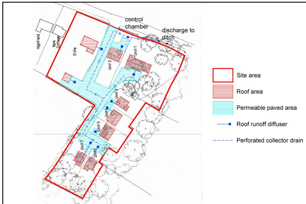
Figure 18. Schematic surface water drainage layout.
