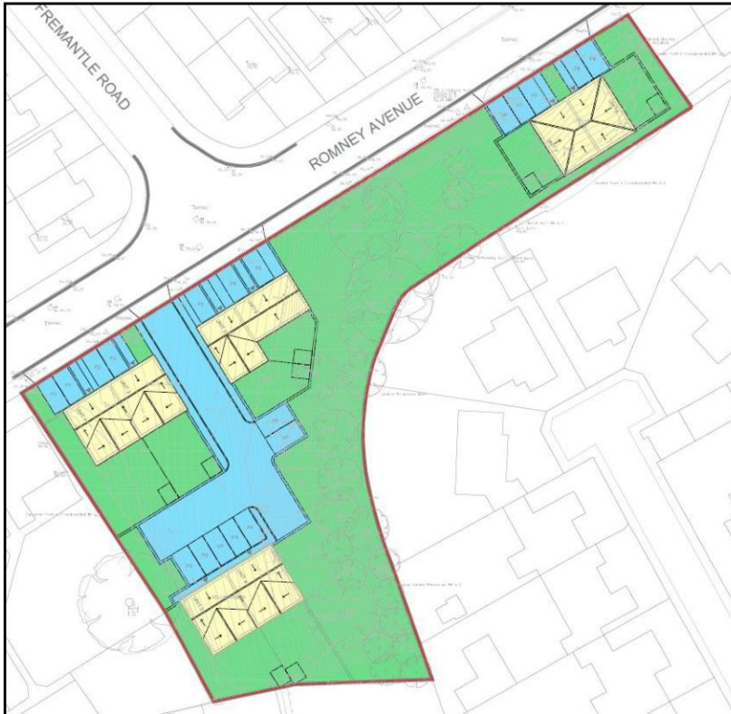
Figure 3.2 – Drained Areas Analysis Extract (Post-Development)
