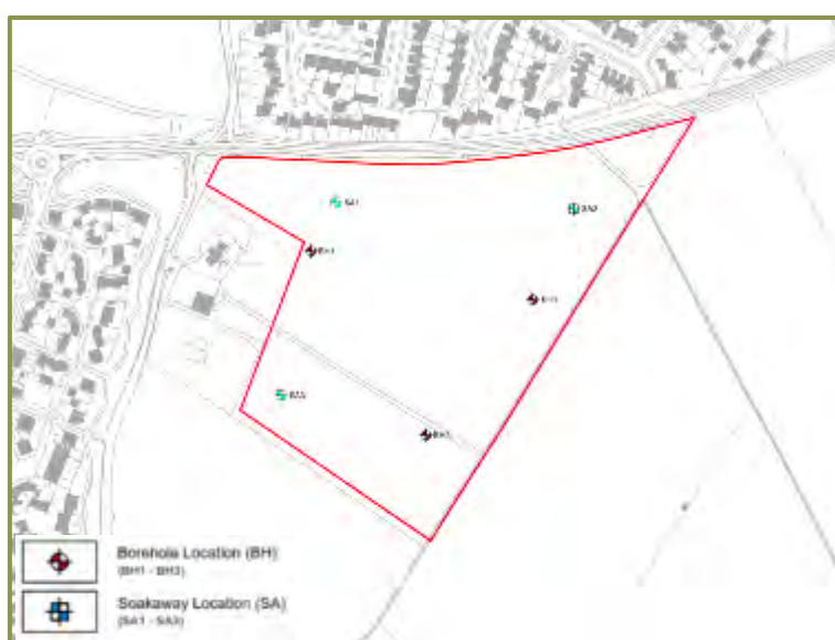
Figure 3.6: Soakaway Test Pit Location
