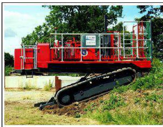
Figure 3.4 – specialist piling rig for steep slopes © TOR Drilling
