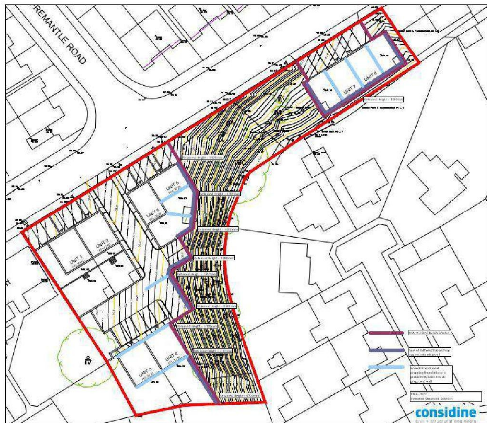
Figure 3.2 – Example of a retaining wall solution - Layout
